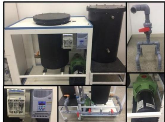
**Figure 2** – Submerged impingement jet (SIJ).
